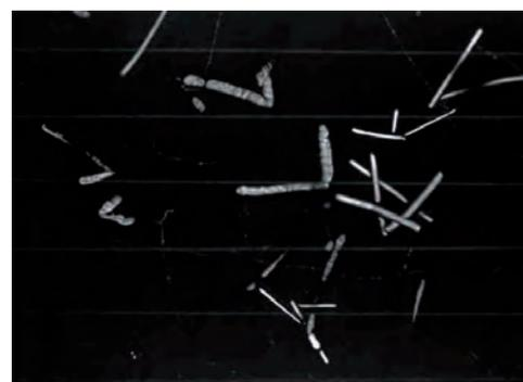
Particles visible in the diffusion cloud chamber.
