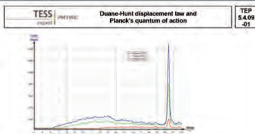
Fig. 8: Bremspectrum of copper for three different anode voltages  $U_A$  (15 kV, 25 kV, and 31 kV), x-axis: glancing angle  $\theta$
