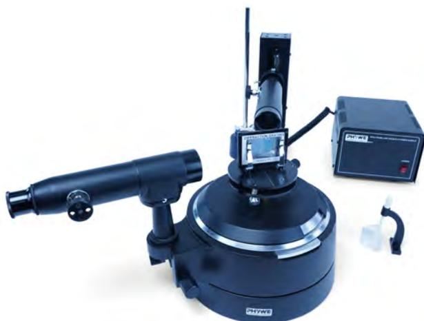
Dispersion and resolving power of a grating spectroscope
